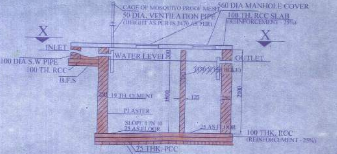
SECTION OF SEPTIC TANK
