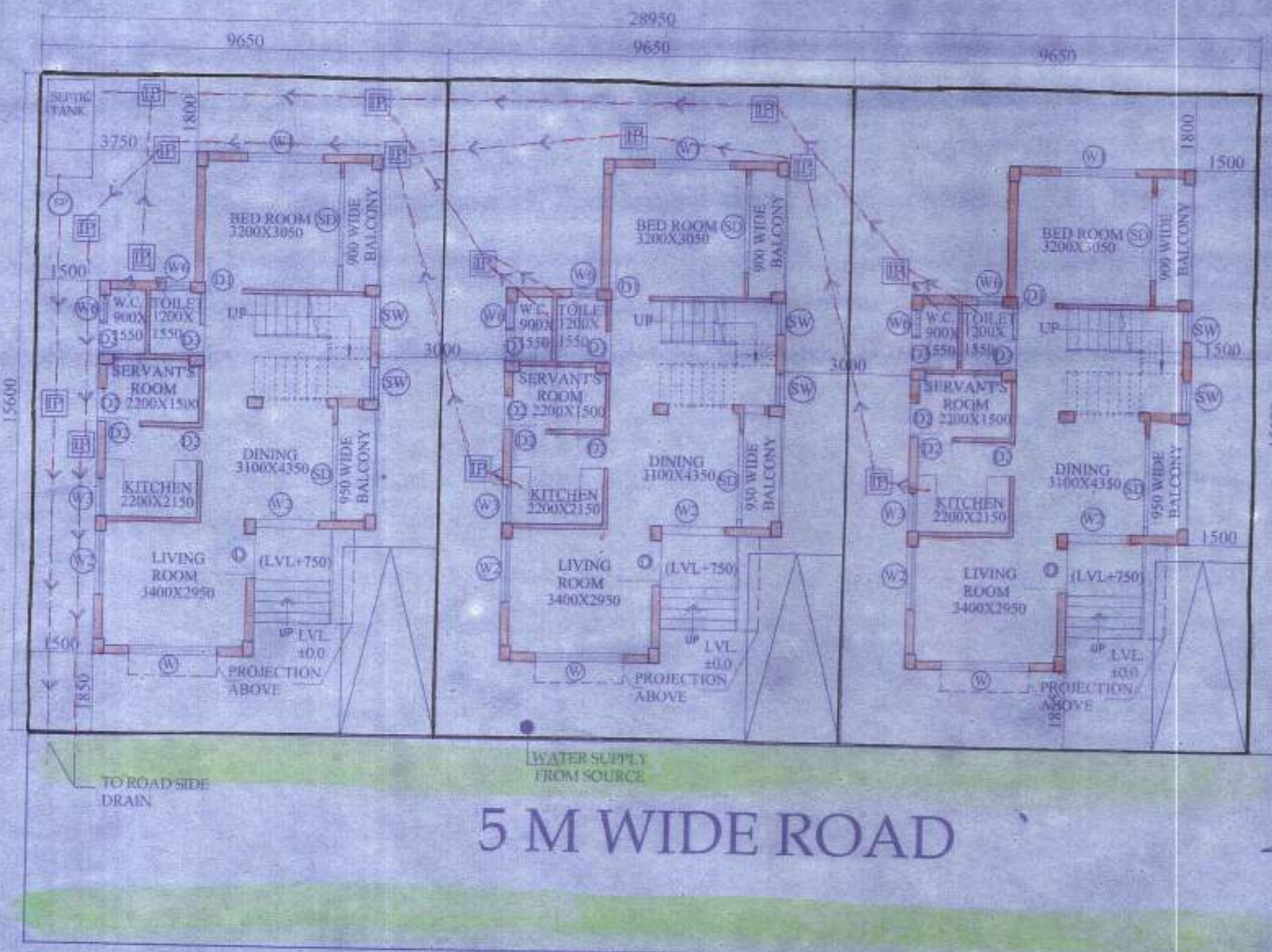
OVERALL SITE PLAN SHOWING GROUND FLOOR PLAN WITH SEWERAGE LAYOUT
